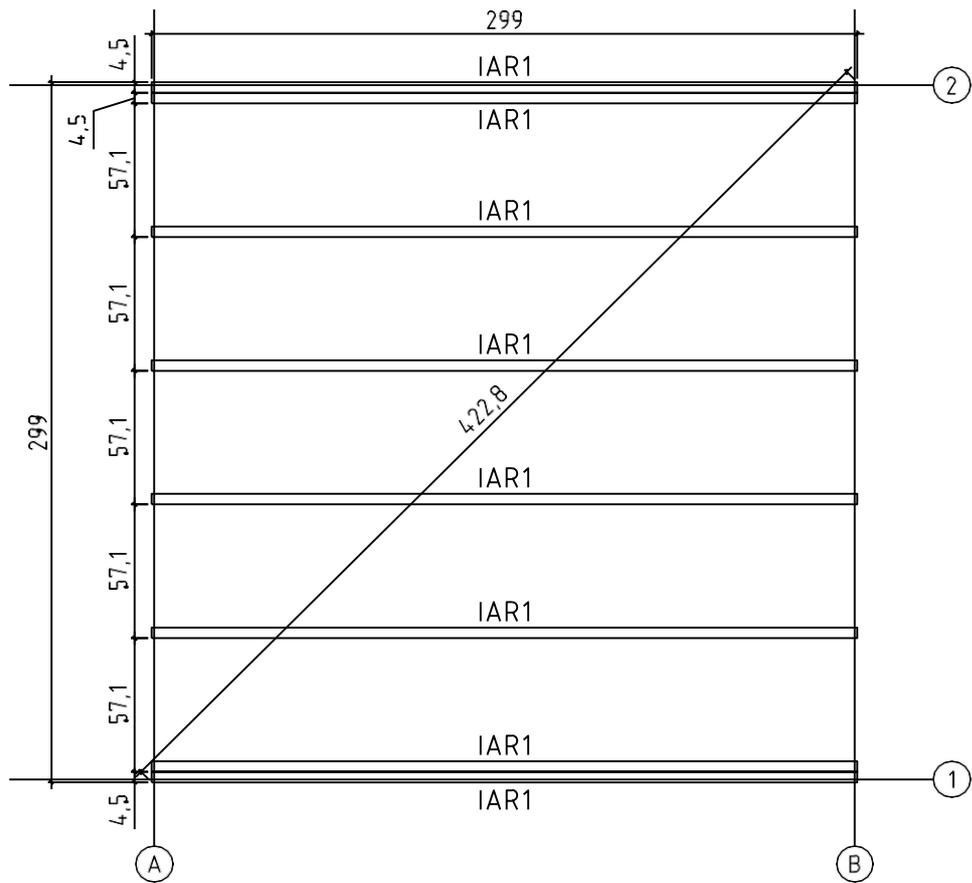
Floor boards - Fussbodenbretter - Plan pose plancher - Pavimento -
